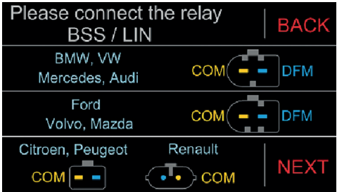
Fig. 10. Graphical symbol of COM terminal location in most common terminals of voltage regulators
