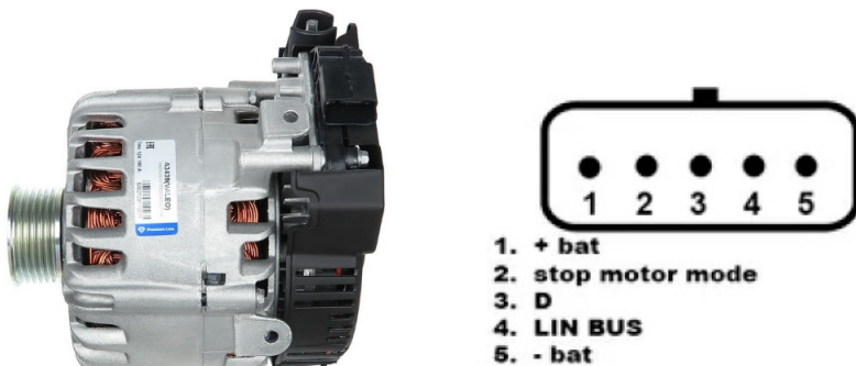
Figure 25. Valeo IST60C017: marking of terminal pins
